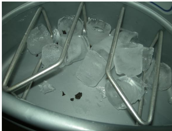
Picture 4: Dirty ice machine nozzle causing black particles in the ice
