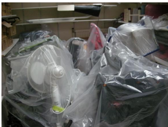
Picture 5 Green trigger tape and plastic sheet covering clean stored equipment
