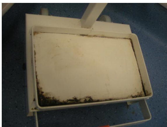
Picture 4 Rusted base of household waste bin
