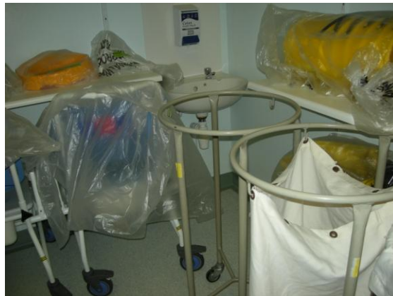
Picture 5 Access blocked to hand washing sink in dirty utility room
