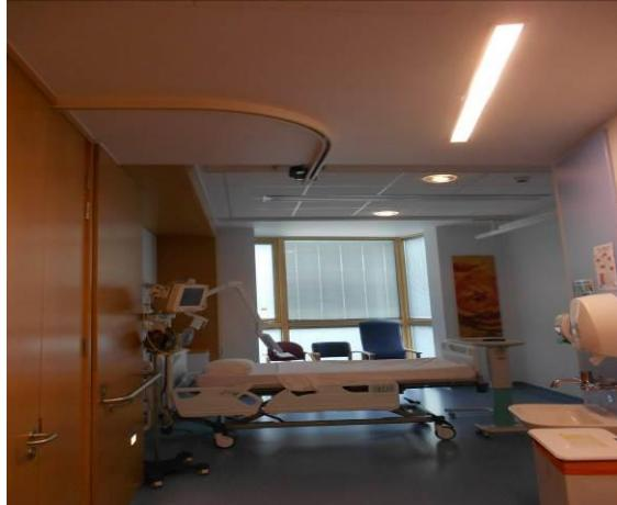
Photo 4 Example of single room with ceiling tracking for hoists
