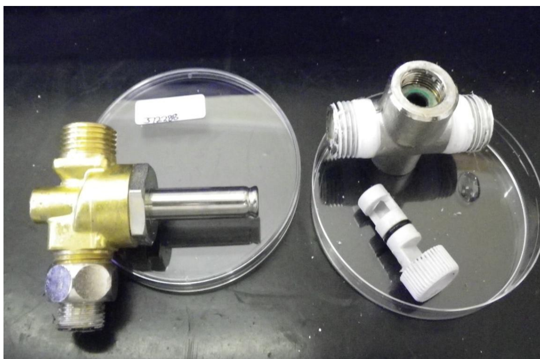
Figure 1.2 and 1.3. Integrated solenoid and blending valve from The Royal Jubilee Hospital, Belfast.
