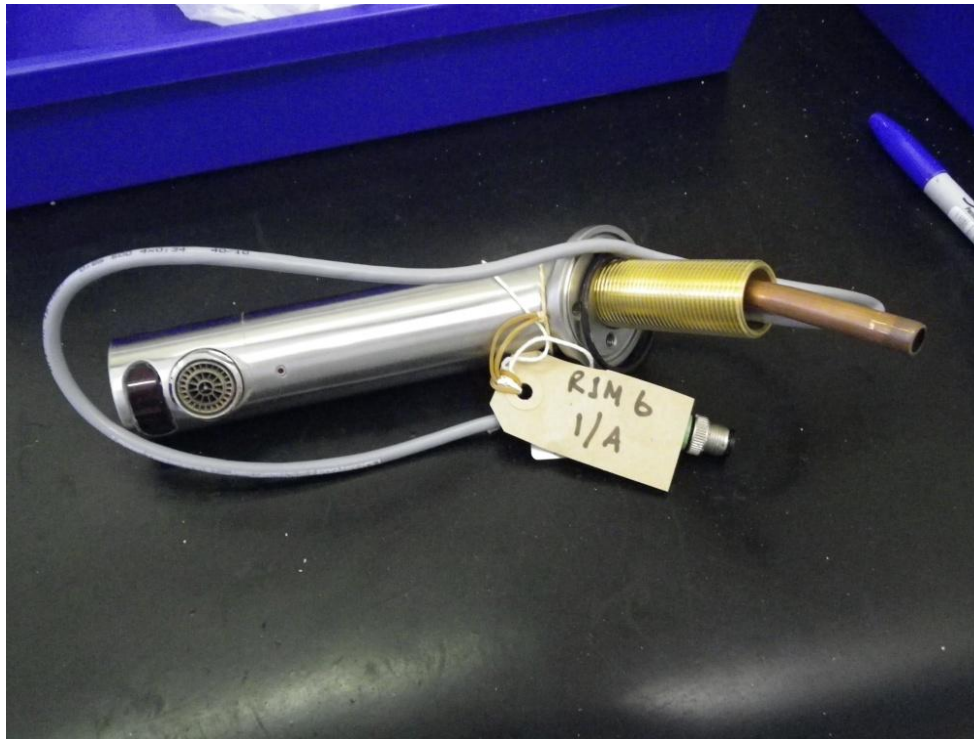
Figure 1.1. Tap assembly with plastic flow straightener in the tap spout nozzle and copper piping from The Royal Jubilee Hospital, Belfast.
