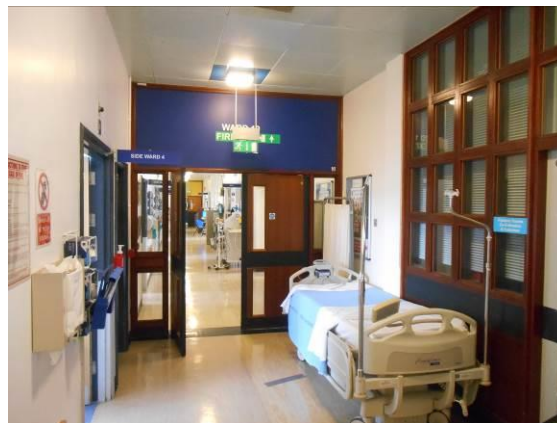
Picture 4 Escalation bed in corridor blocking access to the fire exit
